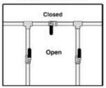
Above is a generic three valve bypass diagram. This will allow service of the pressure booster system when ball valves are set as shown above in the "Bypass Position" configuration.
